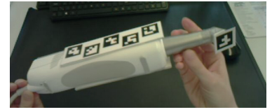
Figure 6: Scanner with an additional marker at the tip (the coordinate system origin) during image acquisition for SfM.
